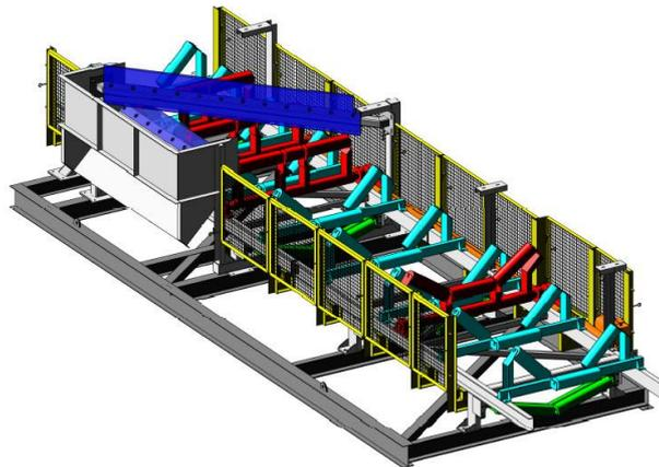
The H & B conveyor diversion plough (plow) was developed & is used to create a secondary circuit on any fixed mining conveyor. It can remove or divert any unwanted material from a carry belt.
