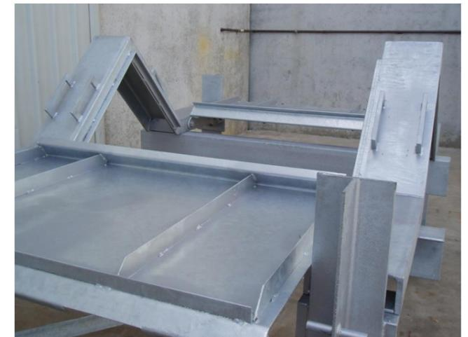
**DUST COVERS FULLY OPENED AND RESTING ON DUST COVER SUPPORTS. FLAT COVERS ACT AS A W/WAY AND PLATFORM TO AID WITH ACCESS FOR INSPECTION AND MAINTENANCE**
