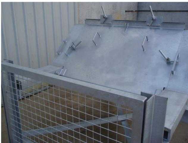
**D.I.L.O GUARD FITTED BETWEEN DUST COVER SUPPORT POSTS - DUST COVER IN CLOSED POSITION**
