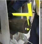
EMRI Belt Change-out, Blocked Chute Clean-out Position
