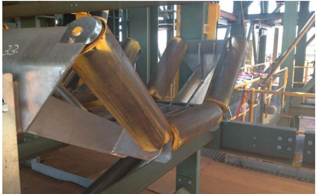
The 'Easy Maintenance' drop down conveyor idler provides a quick, easy, safe and economical way to change out worn or damaged idler rollers on a mining conveyor.
