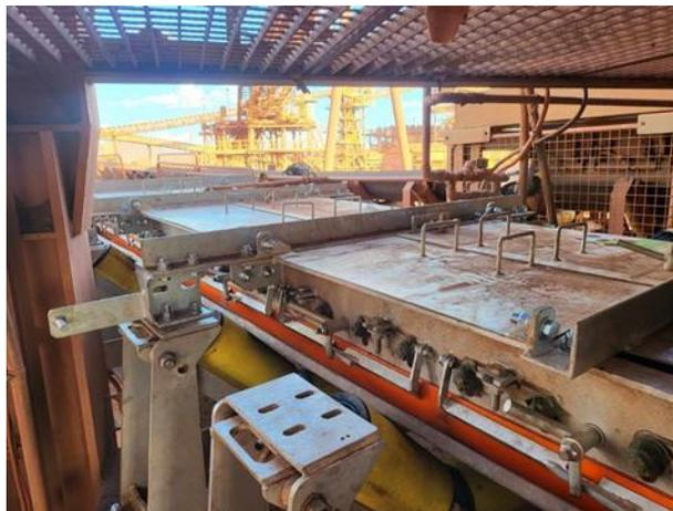
The 'Streamline' conveyor transfer design eliminates the need of any secondary support steelwork normally required to hold up conveyor skirts, dust covers and conveyor guards.
