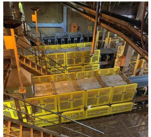
Post-less Guards provide 100% access to all consumable skirt & idler components including idler rolls, skirt liner & skirt rubber. The post-less conveyor guard system utilises the EMRI (Easy Maintenance Retractable Idler) as a support mechanism for the guard.
