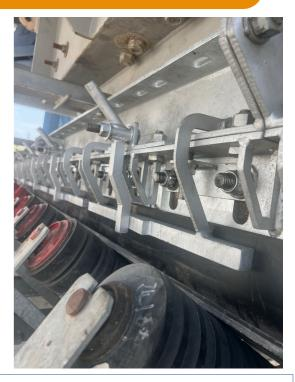
Segmented Ultraseal Skirting features segmented skirting panels which allows access to skirt liners for liner change-out without having to climb on the belt. This skirt design includes a smart clamp to hold the ultra-seal soft skirt in place.
