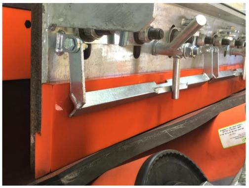
The Ultraseal skirt is designed from 12 thick plate making it the strongest skirt on the market. It is lined with either Ni-hard liners or studded Bissalloy liners; both allow for vertical adjustment of skirt liners externally. The skirt liners can be adjusted vertically up 25mm and down 30mm, this feature allows for better containment of material whilst also extending the life of the skirt liner.
