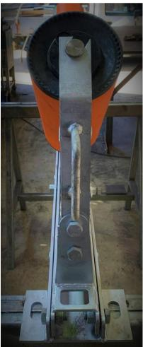
H & B Mining's RRC-EMRI provides a solution to a long-standing issue; how to complete roller changeout when a conveyor only has access on one side.
