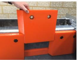
The skirt liners can be designed to replace a minestandard liner and can be manufactured from a material of the mine's choice.
