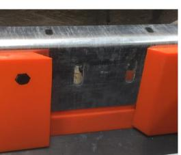
The sloping vertical edges of the liner encourage material flow along and underneath the liner. The 'Better Flow' skirt liner will significantly reduce belt wear if not completely eliminate it.
