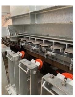
Shut down time for chute maintenance can be massively reduced on multiple feed conveyors by incorporating H&B's Speilbar (False Deck) design.
