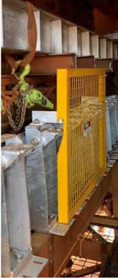
The H & B Mining post-less guarding system provides unrestricted access to all consumable skirt & idler components including idler rolls, skirt liner & skirt rubber.
