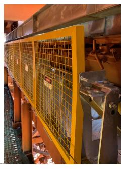
extended base plate of the EMRI. The studs are supplied with hex nuts to lock the guard in place. A simple, modular, maintenance-friendly, robust guarding system.
