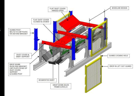
The 'Streamline' conveyor transfer design is a self-supporting system which utilises the idler end brackets as common supports from which all conveyor skirts, dust covers and guards are supported. This innovative design creates 100% clear and safe access to all areas around the conveyor transfer.
