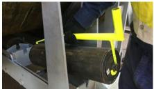
The Rack'n'Roll is a portable rack designed to be mounted on standard hand rail panels in which idler rolls can be mounted in readiness for roll change out. Utilising the rack'n'roll for roller change out offers a hands-free procedure which is simpler, safer and quicker.
