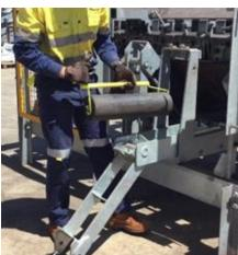
H & B Mining's patented roller removal tool is used to lift the roller from the rack and into the lowered frame of the EMRI. The roller removal tool guarantees that the slot in the roller shaft remains vertical allowing for the roll to be dropped into place between the EMRI roll support plates.
