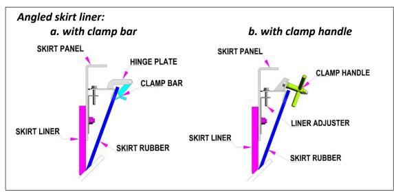
The H & B 'Easy Maintenance' conveyor skirting system allows for simple, quick and safe maintenance of skirt liners, resulting in minimal spillage and material build up around conveyor transfer areas.
