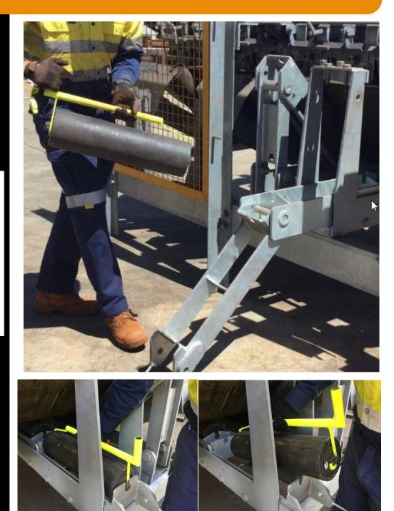
The H & B Mining patented Roller Removal Tool has been designed to enhance roller removal and replacement in conjunction with the EMRI (Easy Maintenance Retractable Idler).
