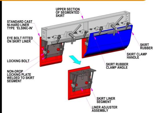
The H & B segmented conveyor skirt design has three innovative features:
