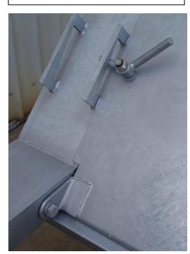
DUST COVER HINGED TO DUST COVER SUPPORT WITH A REMOVABLE PIN
