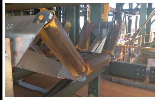
The 'Easy Maintenance' drop down conveyor idler provides a quick, easy, safe and economical way to change out worn or damaged idler rollers on a mining conveyor.
