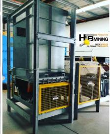
The EMMTT (Easy Maintenance Model Training Tool) assists site personnel to better understand how H & B's easy maintenance conveyor products operate; and how they can be maintained to make transfer points safer and more productive.
